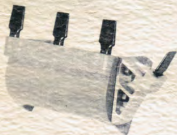
Bucket showing extension socket for 18" cut.
